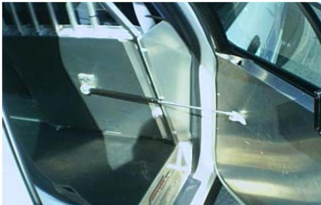
Gas Spring installation photos from a Ford Crown Victoria. The door is opened wide allowing ample room for the K-9 to exit. Mount directly to door frame with supplied bolts, nuts & washers. The mounting ball is removable so the door cover can be cut professionally.
