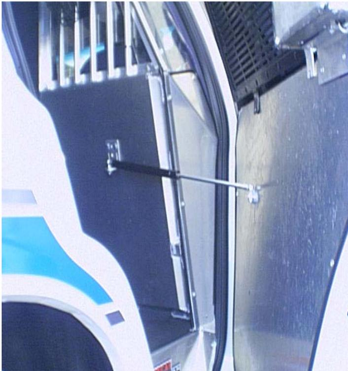
With the door skin removed; enter the vehicle and close the door that you are attempting to open with the gas spring. Position the closed spring on the floor of your cage and examine which location is most suitable for attaching it to door.
